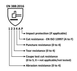
X: indicates that the glove has not been tested
